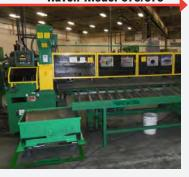
The Haven Tube Cutters are highspeed cutoffs that use a double cut process to re-cut tubing from mill lengths to customer-specified shorter lengths. With the Haven, there are no metal shavings to be removed after cutting. The end condition of the tubing after cutting is dimple-free with minimal burr.
