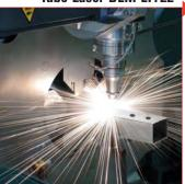
This is a complex machine that can cut and/or etch designs into tubular and open shape products. The laser is not limited to holes, slots and/or straight end cuts. There is no hard tooling involved in running products so this opens up the possibilities of shorter runs that can be cost effective
