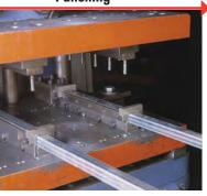
Allied has punch presses ranging in size from 10 tons to 125 tons. Tubular applications of the punch press include: piercing, notching, flattening, coping, punching, slotting (with or without a mandrel) and specialty re-cutting. Flat stock and plate can be stamped to produce brackets and fittings.
