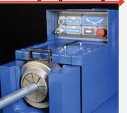
The large segment swager can swage round tubing as large as 5.000" OD, and as heavy as 8 gauge. On a segment swager, the die opens to the size of the mother tube, then squeezes the tubing down to a specific dimension. During the swaging process, some minor ridges are formed on the swaged area.
