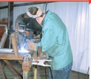
Capabilities include MIG and resistance welding of tubing and plate stock to produce custom parts
