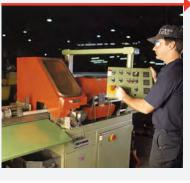
There are two Scotchman cold saws currently in use at Allied. The primary function of these saws is to cut heavy wall tubing, especially cuts with a tight length tolerance. The Scotchman saws provide precise tolerances and leave a minimal burr. Our cold saws are also capable of cutting steel bar or rod at any angle up to 90°.
